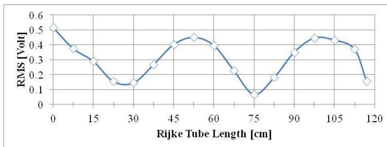
Third mode of the tube  $n=3$  ( $f=370\text{Hz}$ )
