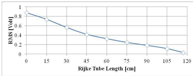
First mode of the tube  $n=1$  ( $f=74\text{Hz}$ )
