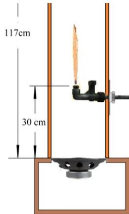
**Figure 11: Burner position in the Rijke tube.**
