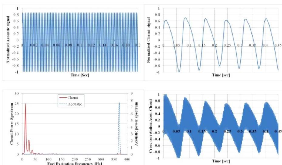
**Figures 21: Normalized acoustic and chemiluminescence emission signals, power spectrum and cross-correlation at the third mode of the tube (370Hz) with fuel excitation ( $f=195$ Hz).**
