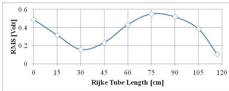
second mode of the tube  $n=2$  ( $f=222\text{Hz}$ )
