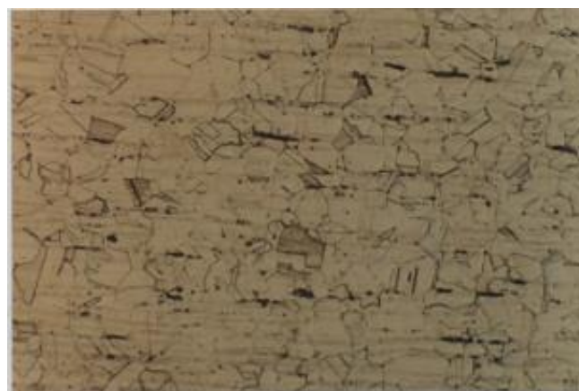
Fig. 2 Microstructure of the base metal after sensitization annealing and streicher test – 200X.
