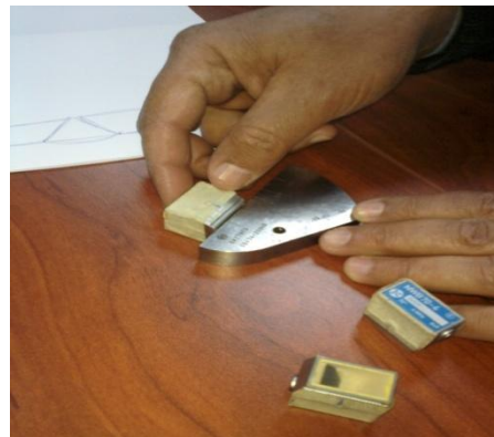
Figure 8. Ultrasonic test prob calibration.
