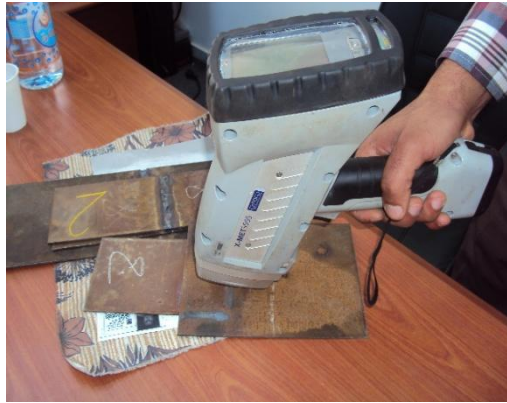
Figure 4. Metallurgy test by a spectrophotometer device (X-MET5000).
