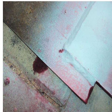
Figure 3. Penetrant test for the sample welded by wet electrode.
