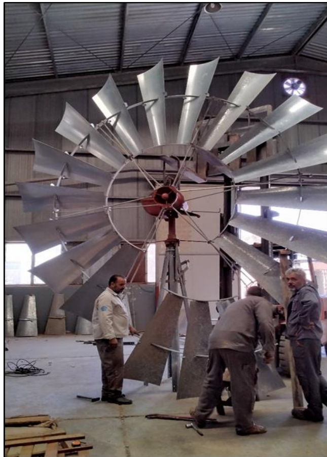
Figure 3-66. Installing the 6th Sails section.
