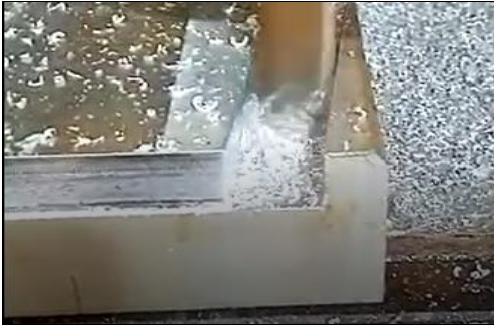
Figure 3-47. "Z-level" operation of lower Sail die.
