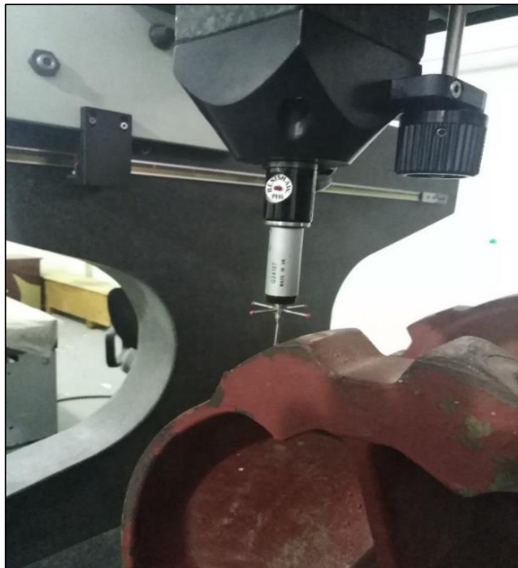
Figure 3-19. The Hub points acquisition using CMM.
