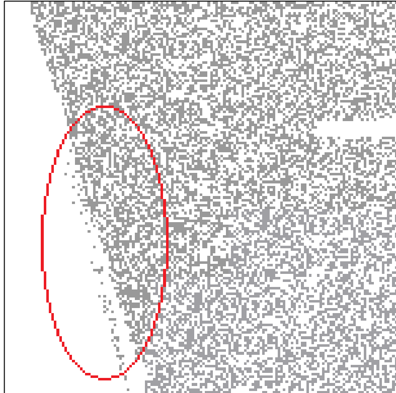
Figure 3-11. Surface color cause incorrect scanning.
