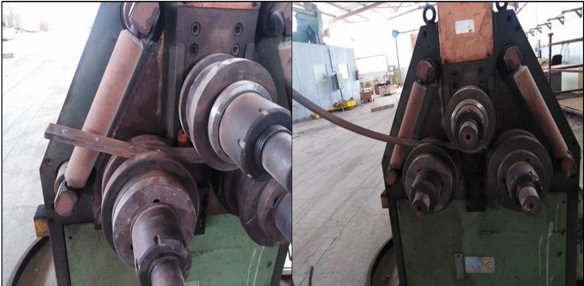
Figure 3-59. Bending the outer Band by CNC rolling machine.
