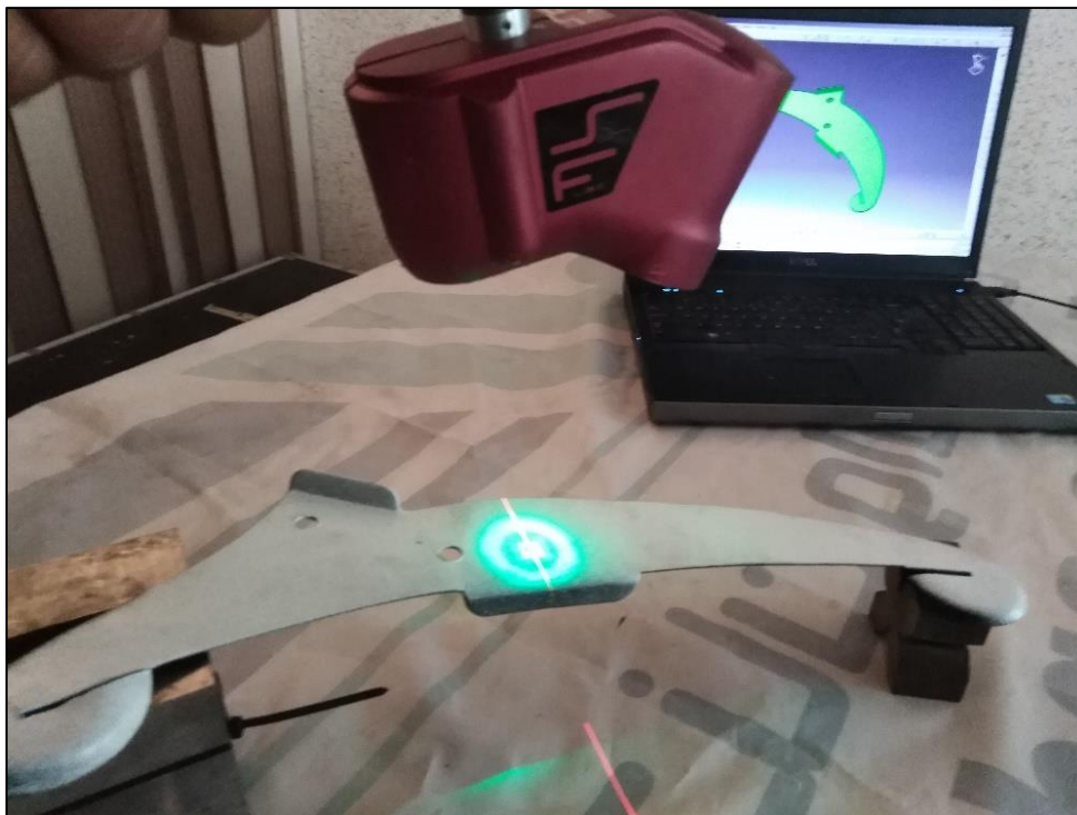
Figure 3-13. The Baces3D arm during scanning of the Sail Rib.
