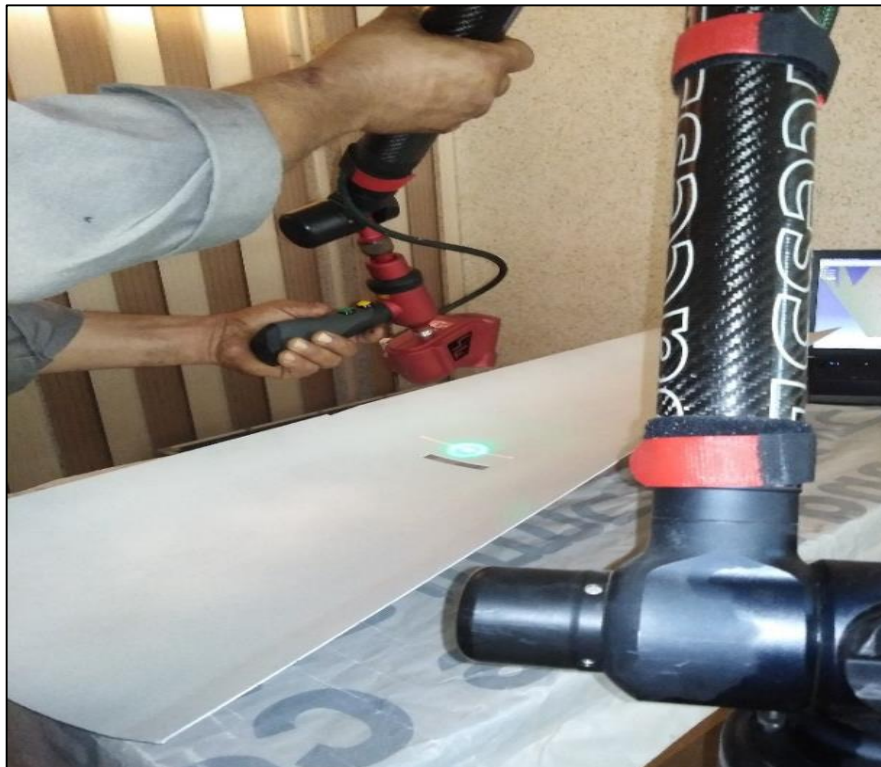
Figure 3-8. The BacesSCAN laser scanning system is shown in a moment of its use.
