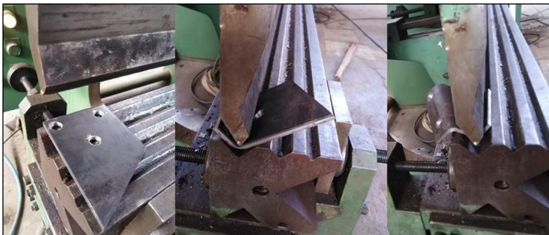
Figure 3-55. The bending process of the Sail Tie by the bending press machine.
