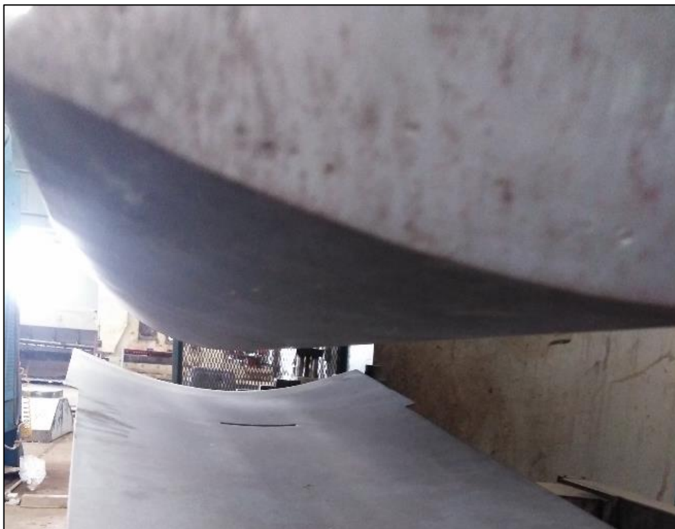
Figure 3-49. Sails curving die installed on the bending machine.
