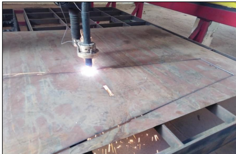
Figure 3-51. Cutting the Sails using a CNC plasma machine.
