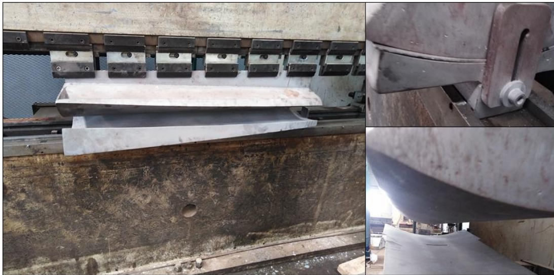
Figure 3-52. Curving Sails die attached to the bending machine.
