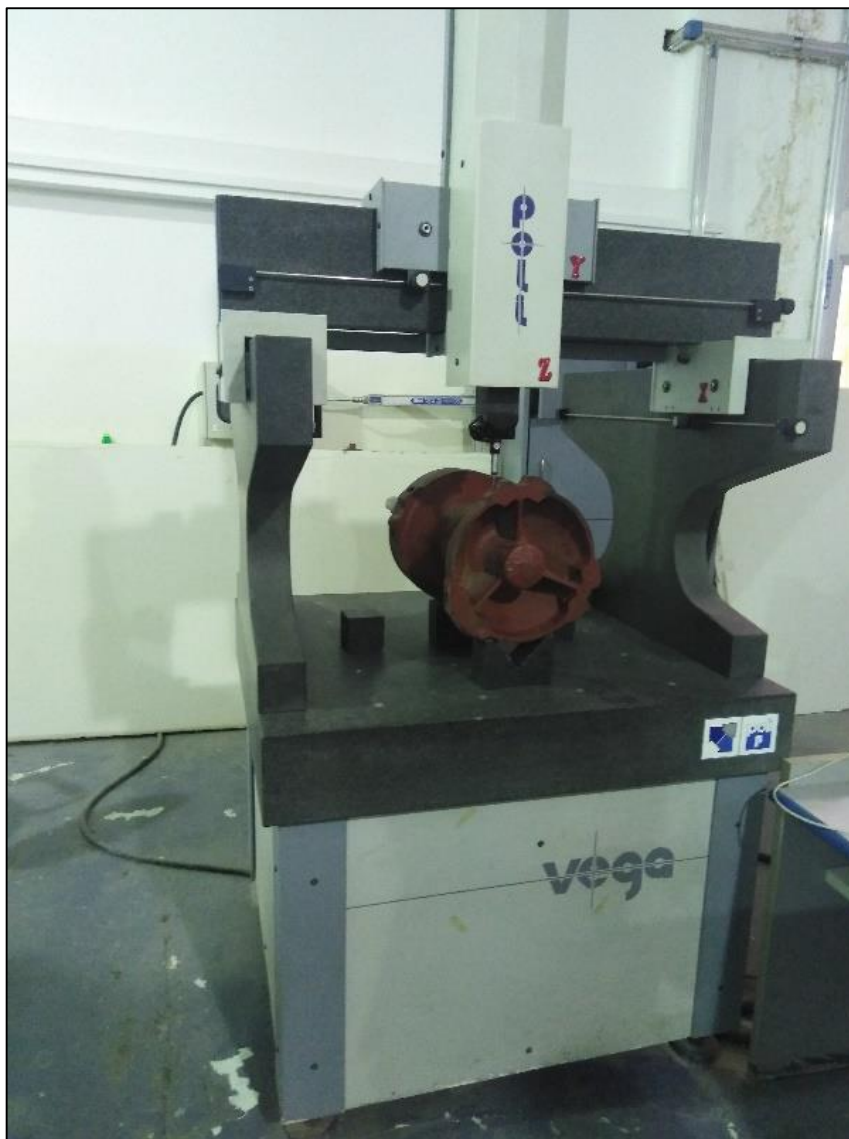
Figure 3-9. CMM during some measurements of the Hub.
