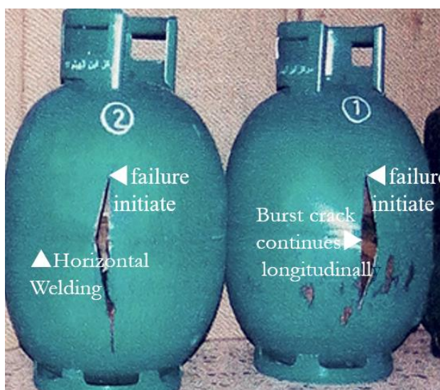
Fig. 6. Showing the Crack Shape, Length and Position Relative to Welded Region
