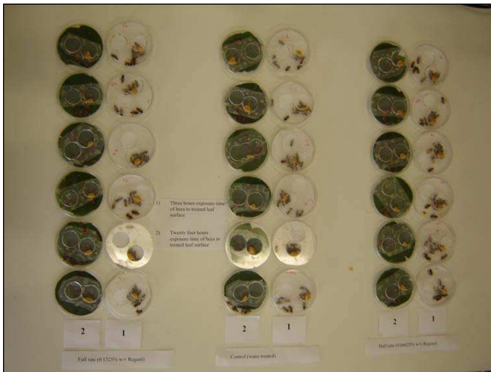
Figure 6.2 Experimental setup for assessing toxicity to honeybees of fipronil residues on cotton foliage exposed to normal weather conditions. Petri dishes labeled 1 contain bees which had already been exposed to treated leaves for 3 h, and have been removed to clean dishes. Those labeled 2 contain treated leaves and bees exposed to them for 24 h.
