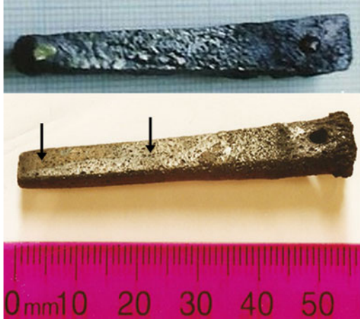
Fig. 1. Optical photographs of Nd(123) melt-processed bars containing single block (top) and multiple blocks (bottom). Arrows indicate blocks.
