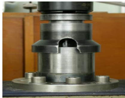
Figure (7): The die set for backward extrusion.
