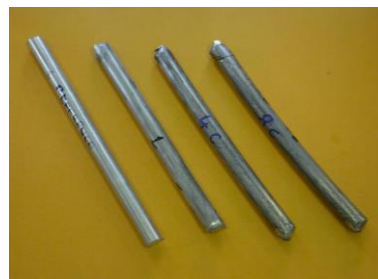
[47] Figure (6): From the left: zero pass, one pass, four passes and eight passes respectively using
