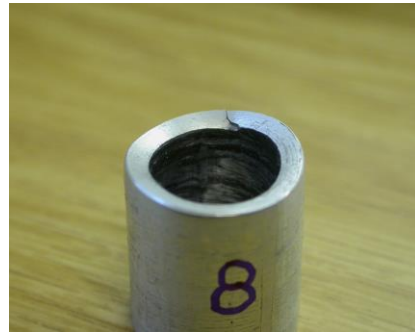
Figure (13): Typical crack on a cup produced by backward extrusion (after eight ECAP passes by route C, and Al-6282 alloy).
