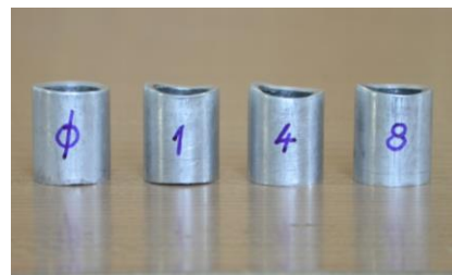
Figure (9): View of backward extruded cups, from left, after zero, one, four and eight passes.
