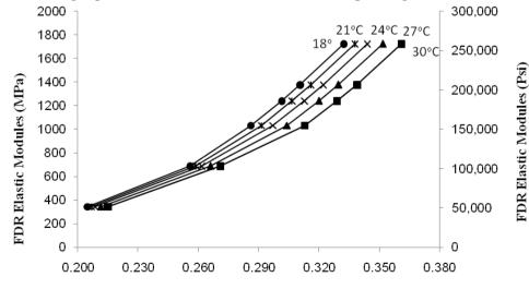
Structural coefficient For FDR Layer Figure 3: the relationship between the FDR modulus and the FDR layer structural coefficient for different MAATs
