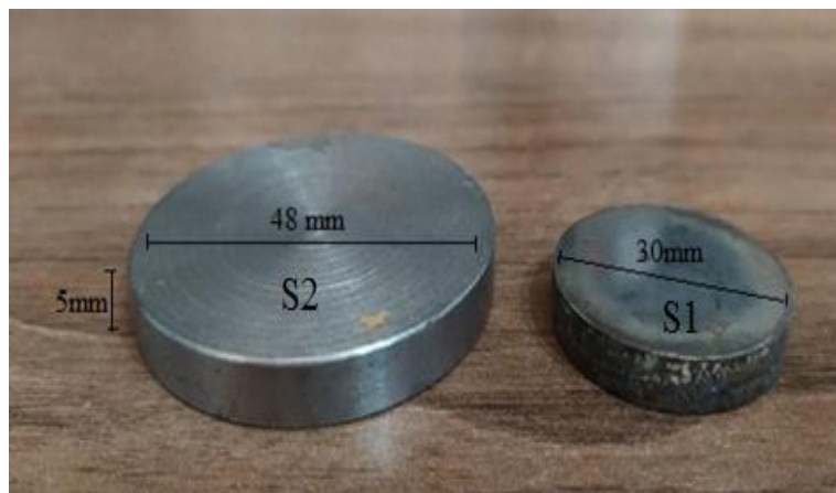
Figure 3.1 As received steel samples
