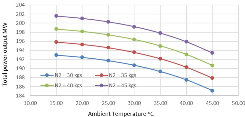
**Figure 4: The power output of the combined cycle with injection of different N<sub>2</sub> mass flow rate as a function of ambient temperature**
