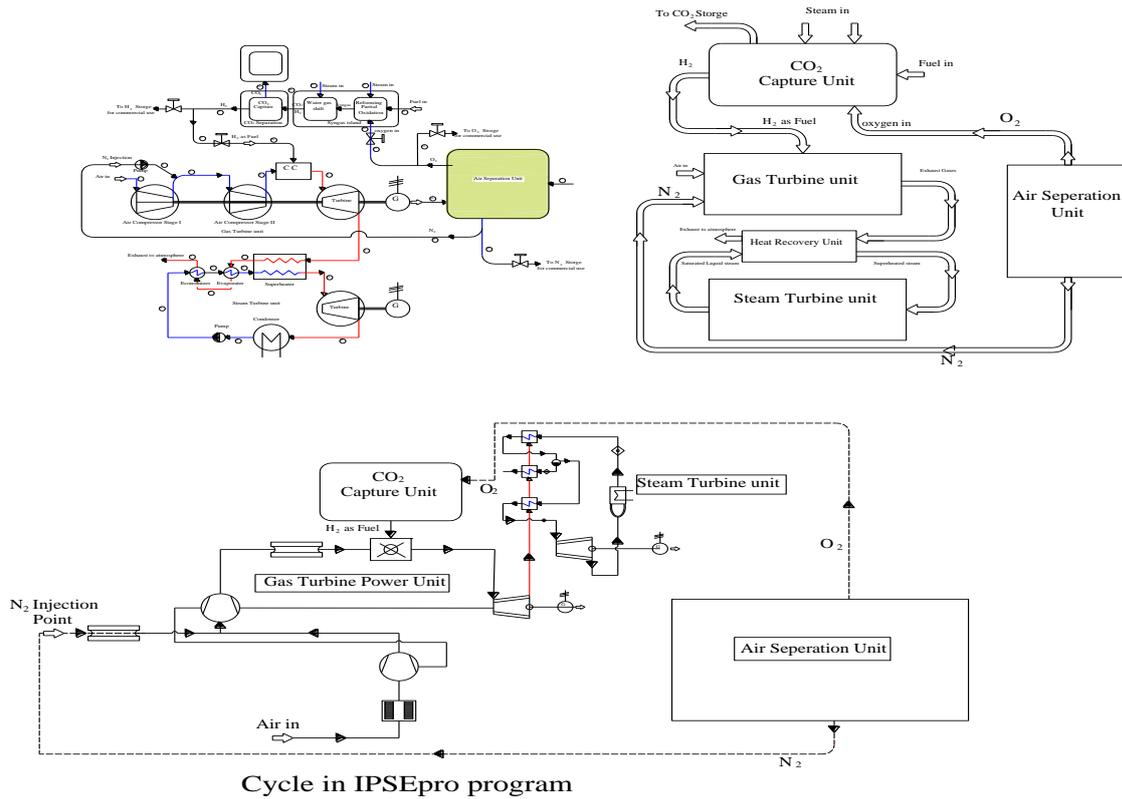
**Figure 3 Pre-Combustion Combined Cycle with N<sub>2</sub> Injection**
