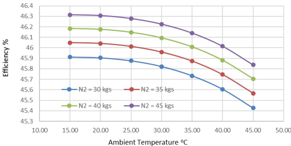
**Figure 5: The efficiency of the combined cycle with injection of different N<sub>2</sub> mass flow rate as a function of ambient temperature**
