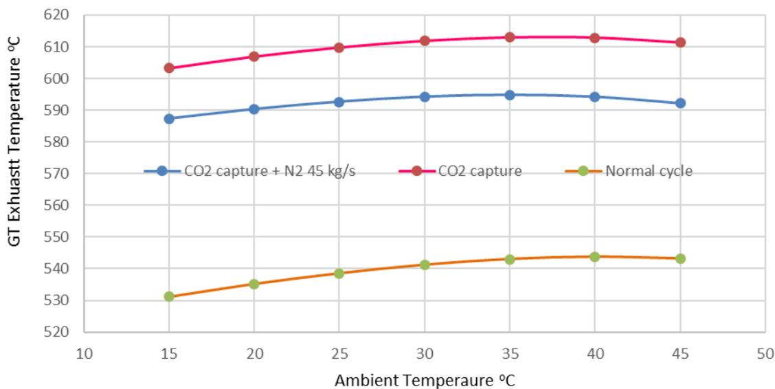
**Figure 10: The gas turbine exhaust gas temperature as a function of ambient temperature for the 3 cases**
