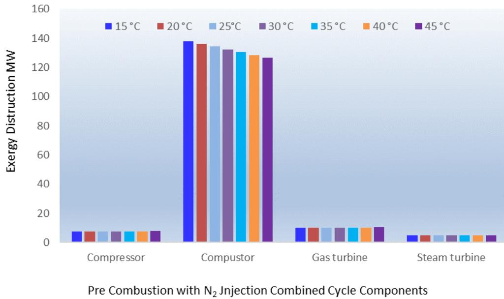
**Figure 9: Exergy destruction of the CO<sub>2</sub> capture + (45 kg/s) N<sub>2</sub> injection as a function of ambient temperature**
