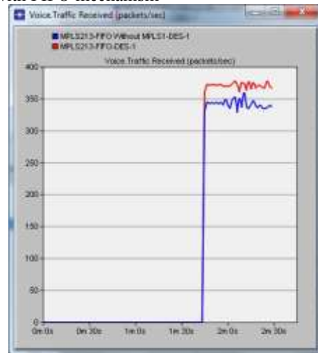
Figure (5): Voice: traffic received (packets/sec) for TCP/IP (Blue) and MPLS (Red) with FIFO queuing mechanism
