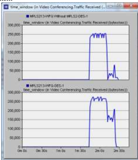
Figure (11): Video conferencing: Traffic received for TCP/IP (UP) and MPLS (DOWN) with WFQ mechanism
