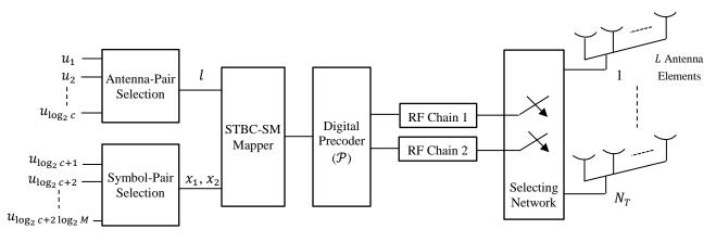
Fig 1. Block Diagram of the Proposed STBC-SM-aided mmWave MIMO Scheme with Hybrid Analog-Digital Beamforming.
