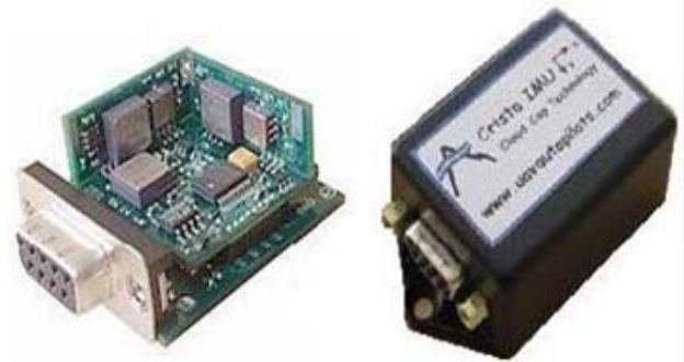
Fig. 6 Cloud Cup Technology Crista IMU which is a very small, low-cost, 3-axis MEMS Inertial Measurement Unit
