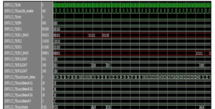
Fig. 19. The timing diagram for the real-time density-based traffic system with road blockage signal.
