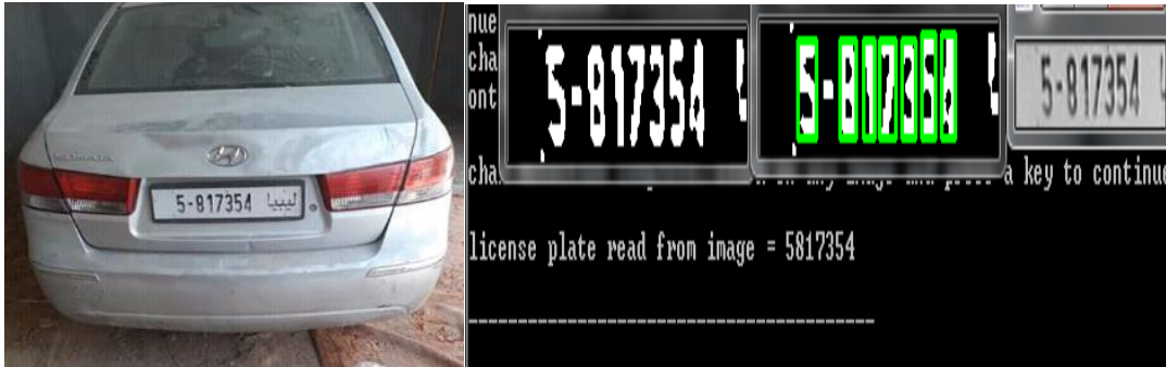
Figure 11(a) image with dust or some oils covering the lower half of the plate, (b) results.
