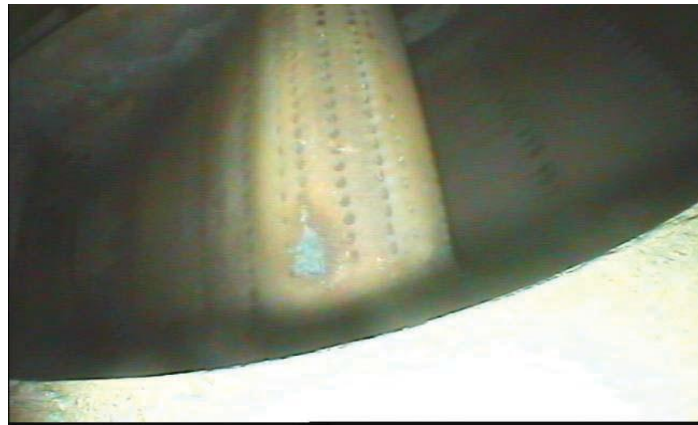
Figure (2.4): Corrosion on the Rise Edge of the Stator Blade of High Pressure Gas Turbine Engine [11]
