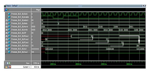
Figure (4.15) The transfer via bus to different registers.
