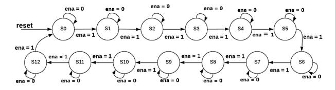
Figure (4.12) Finite State Machine FSM diagram.
