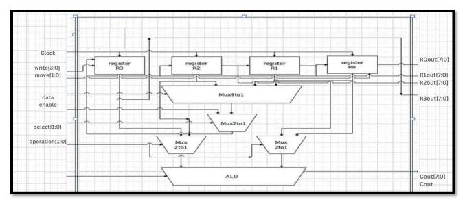
Figure (4.10) MUX top-level schematic.
