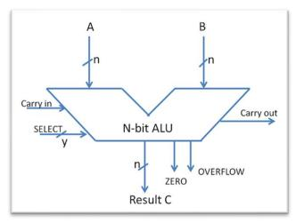
Figure (4.3) Arithmetic Logic Unit.
