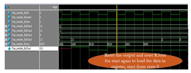
Figure (4.23) Simulation of the top module show executed the operations ADD, SUB, SHL, AND.
