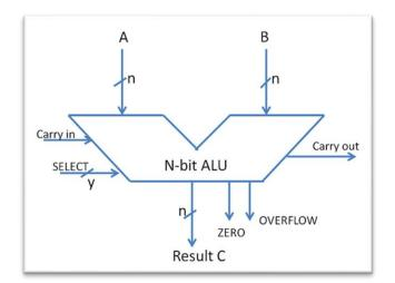
Figure (4.7) Arithmetic Logic Unit.
