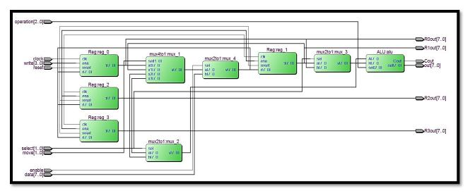
Figure (4.25) Register transfer level schematic for data path MUX 8\_bit.
