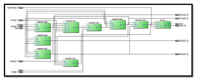
Figure (4.26) Register transfer level schematic for data path MUX 4-bit.
