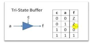
Figure (4.2) Tri-state buffers.
