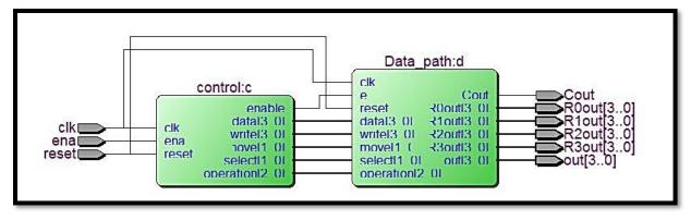
Figure (4.28) Register transfer level schematic for top module MUX.
