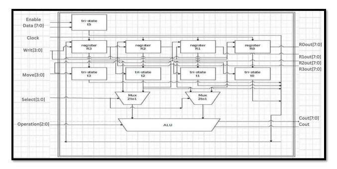
*Figure (4.5) Tri-state top-level schematic.*
