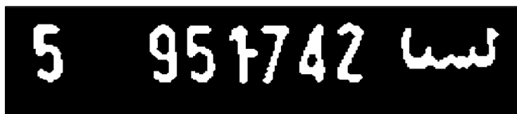
Figure 15: License plate image after removing small objects.
